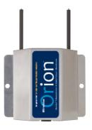
Attach the magnet to the Orion with the supplied 10-32-1/4" screw. You can also use supplied self tapping screws to permanently mount the Orion.
